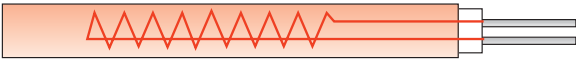
Unbeheizte Zone am Anschluss und/oder Blindende Unheated zone on connection side and/or far end
